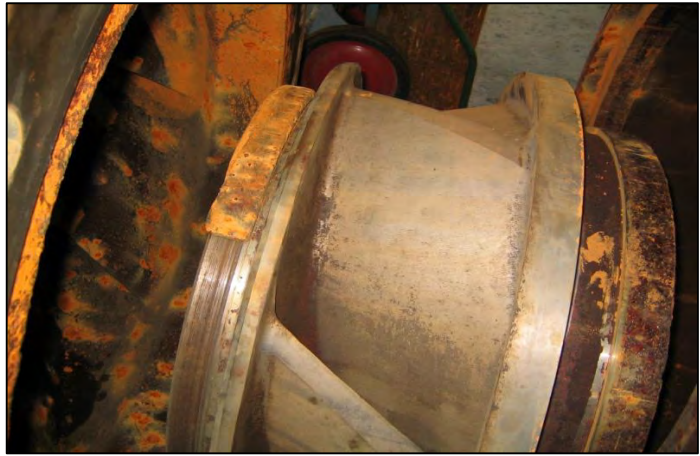
Example of bacterial corrosion on a suction wear ring of an impeller
