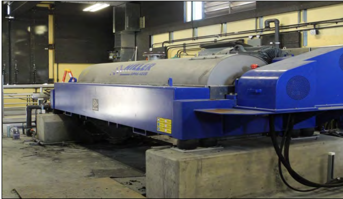
Centrifuge for mechanical dewatering of sludge
