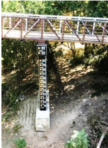
Flood stage gauge at East William Street
