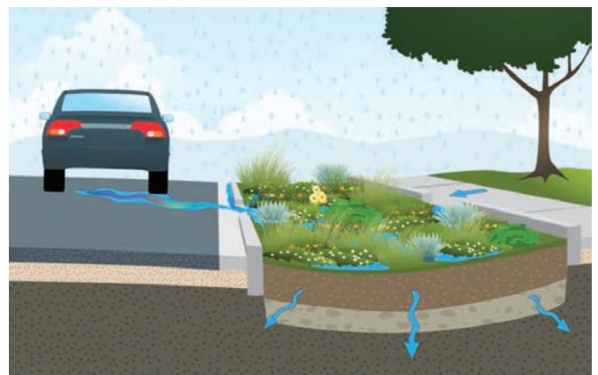
Typical Bioretention Design Green Infrastructure (Image Credit: SCVURPPP).
