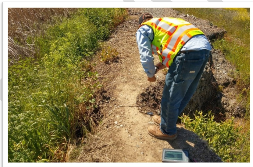
Staff measuring extent of bank erosion along Calabazas Creek
