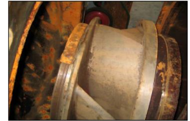
Suction wear ring bacterial corrosion of Impeller. Similar rehabilitation projects will be done in this project.
