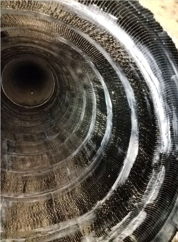
Hoop and Longitudinal Layer of Carbon Fiber
