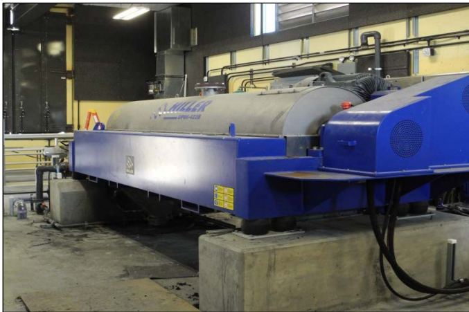
Centrifuge for mechanical dewatering of sludge
