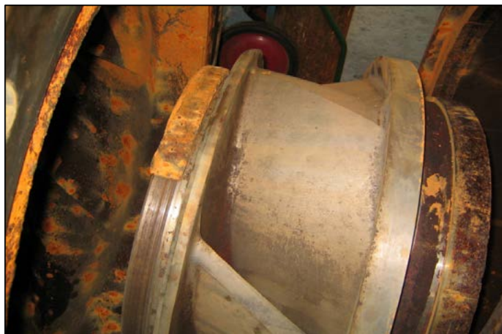
Suction wear ring bacterial corrosion of Impeller. Similar rehabilitation projects will be done in this project.
