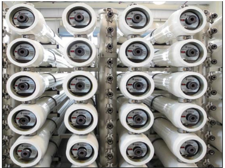
Reverse osmosis membranes used for water purification
