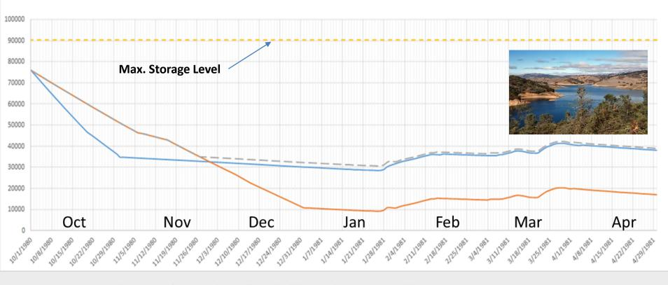
Anderson Storage Level Under Current Operation Curve no pump-over
