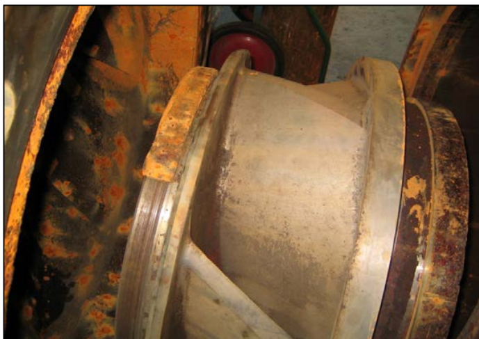
Suction wear ring bacterial corrosion of Impeller. Similar rehabilitation projects will be done in this project.
