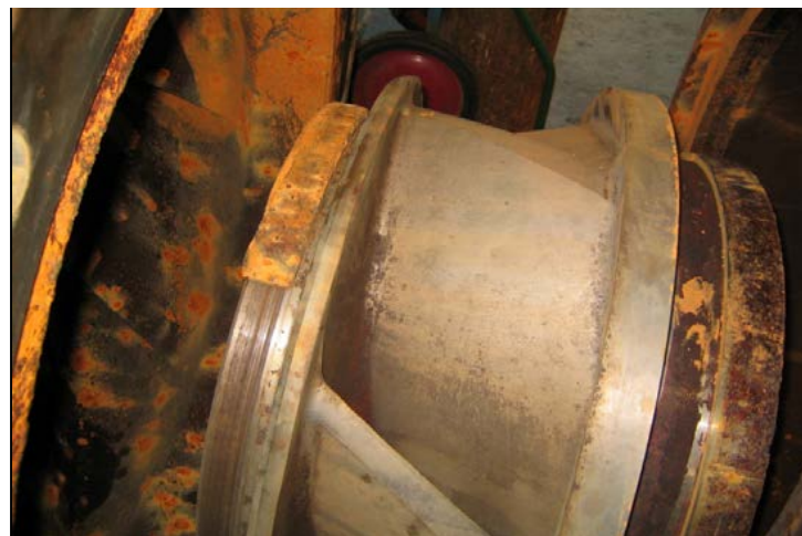
Example of bacterial corrosion on a suction wear ring of an impeller
