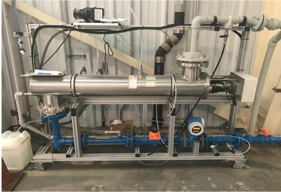
Figure 4. SVAWPC UV/AOP Pilot System
