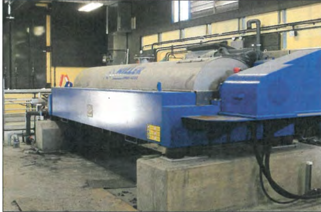
Centrifuge for mechanical dewatering of sludge
