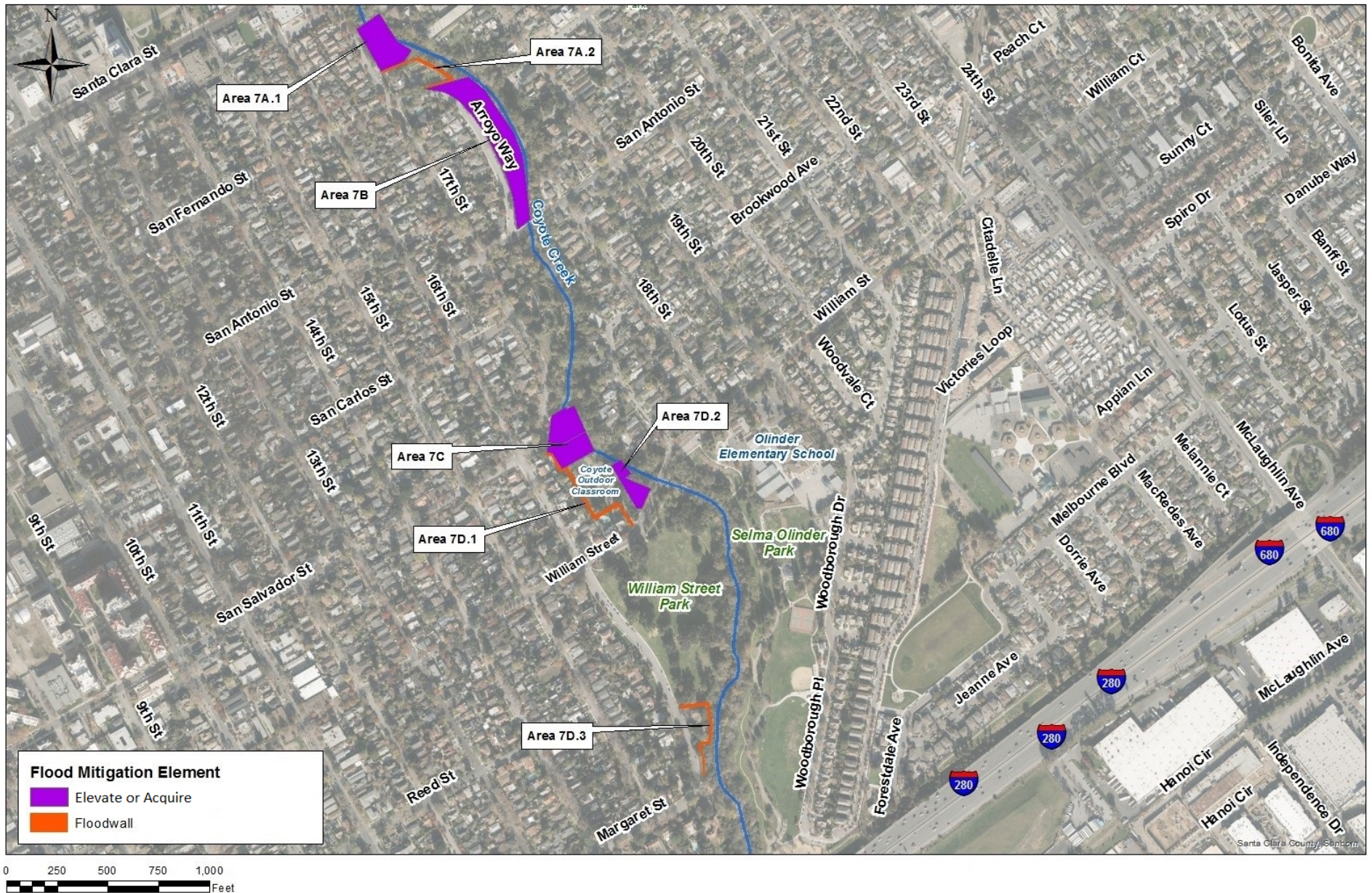
FIGURE 6c. FOCF Coyote Creek Flood Management Measures Site Plan (Reach 7)
