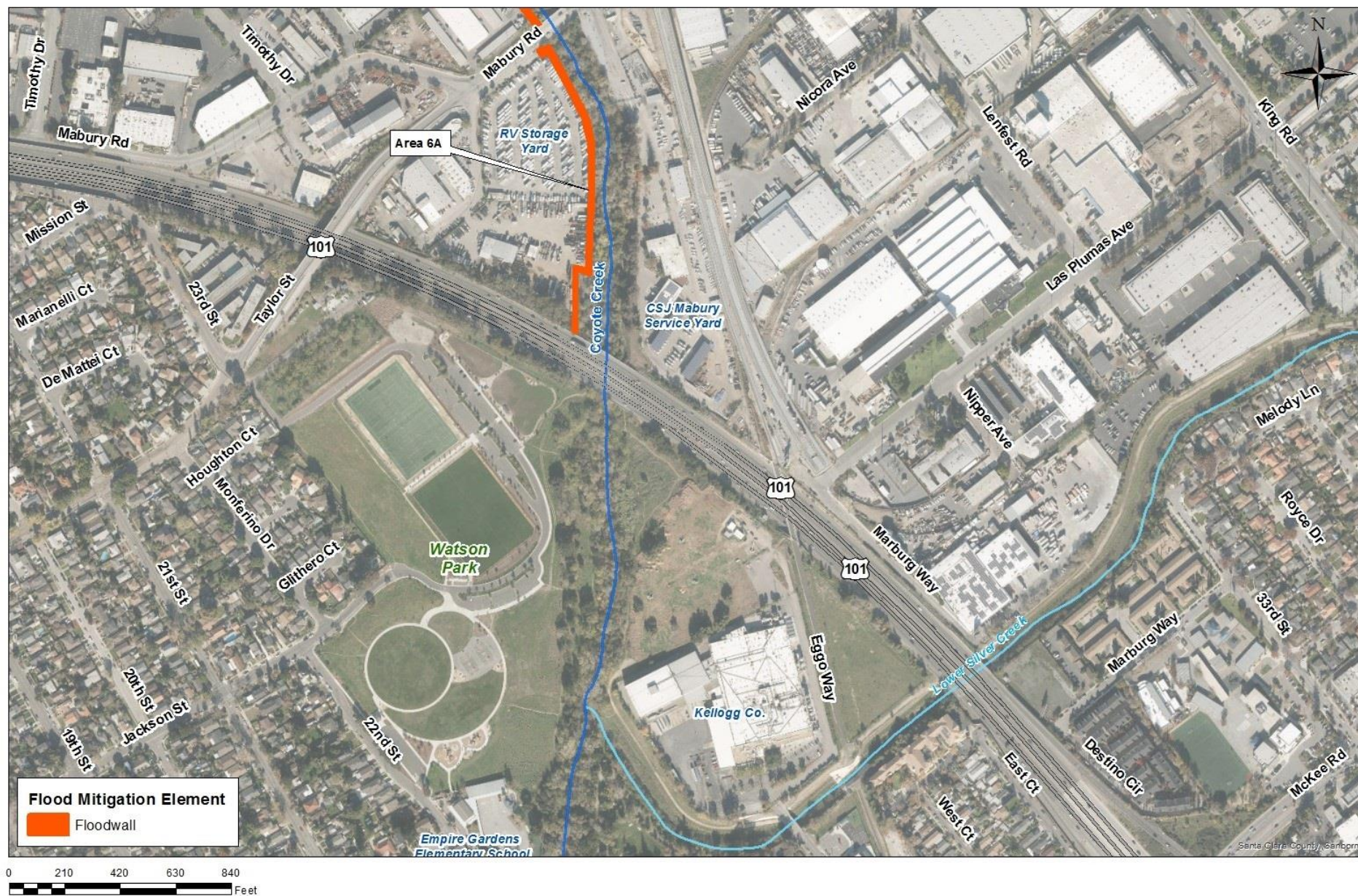
FIGURE 6b. FOCF Coyote Creek Flood Management Measures Site Plan (Reach 6)
