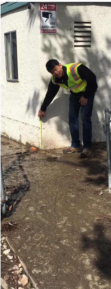
Measuring high-water marks in San José after the Coyote Creek flood of 2017
