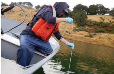
Water column sampling at Guadalupe Reservoir.
